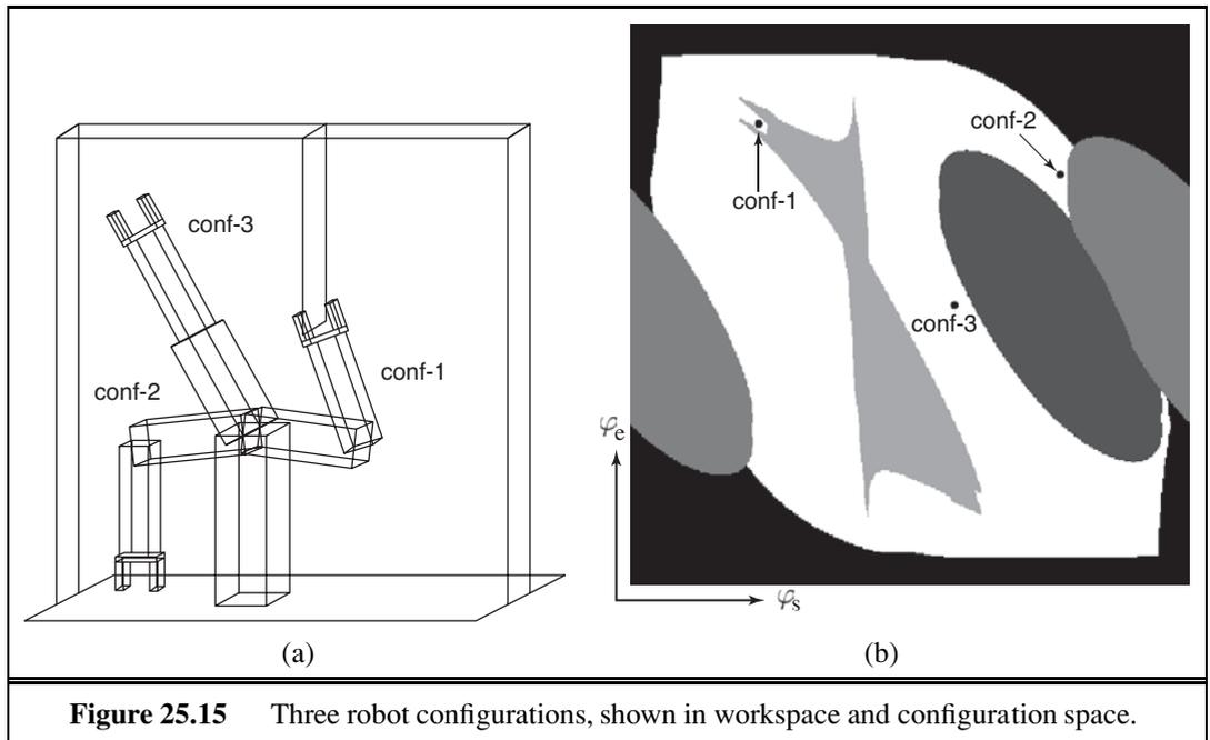
**Figure 25.15** Three robot configurations, shown in workspace and configuration space.
