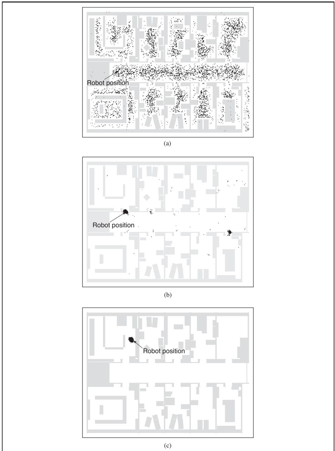
**Figure 25.10** Monte Carlo localization, a particle filtering algorithm for mobile robot localization. (a) Initial, global uncertainty. (b) Approximately bimodal uncertainty after navigating in the (symmetric) corridor. (c) Unimodal uncertainty after entering a room and finding it to be distinctive.
