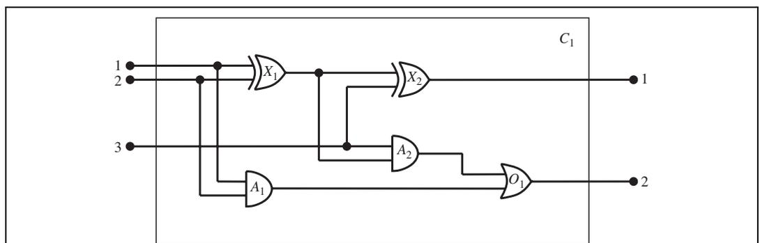
**Figure 8.6** A digital circuit C1, purporting to be a one-bit full adder. The first two inputs are the two bits to be added, and the third input is a carry bit. The first output is the sum, and the second output is a carry bit for the next adder. The circuit contains two XOR gates, two AND gates, and one OR gate.
