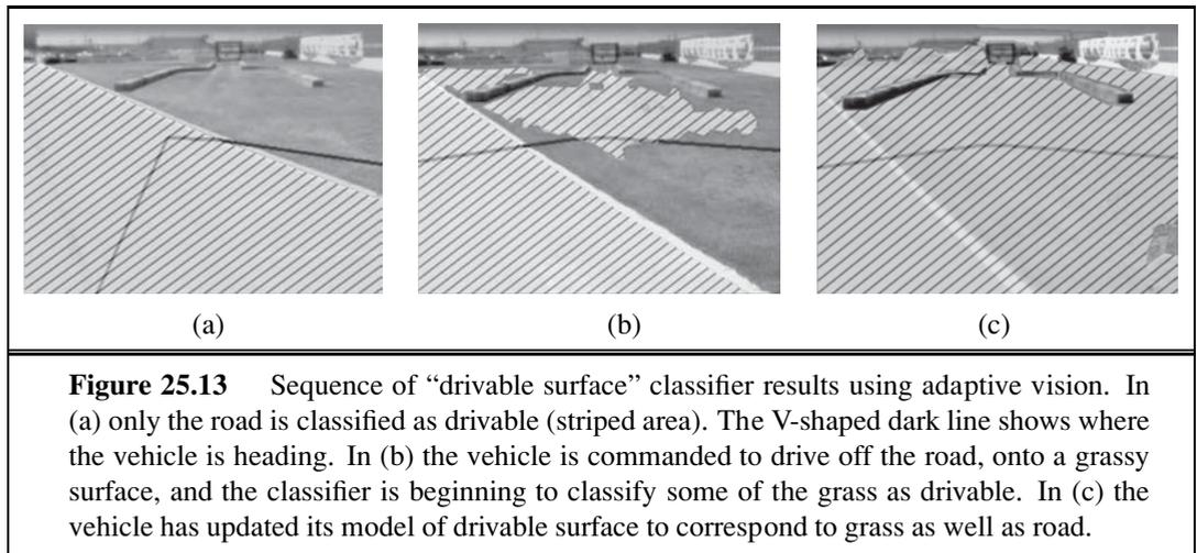
**Figure 25.13** Sequence of “drivable surface” classifier results using adaptive vision. In (a) only the road is classified as drivable (striped area). The V-shaped dark line shows where the vehicle is heading. In (b) the vehicle is commanded to drive off the road, onto a grassy surface, and the classifier is beginning to classify some of the grass as drivable. In (c) the vehicle has updated its model of drivable surface to correspond to grass as well as road.
