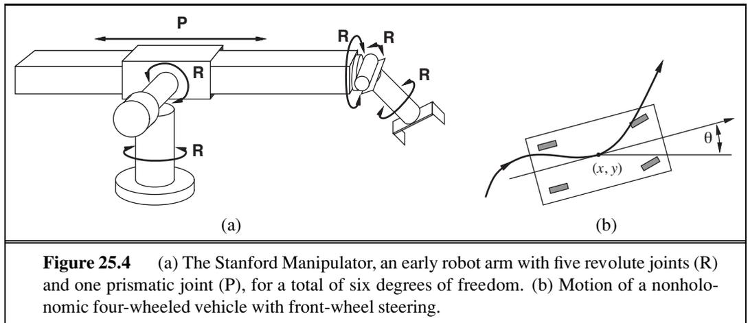
**Figure 25.4** (a) The Stanford Manipulator, an early robot arm with five revolute joints (R) and one prismatic joint (P), for a total of six degrees of freedom. (b) Motion of a nonholonomic four-wheeled vehicle with front-wheel steering.
