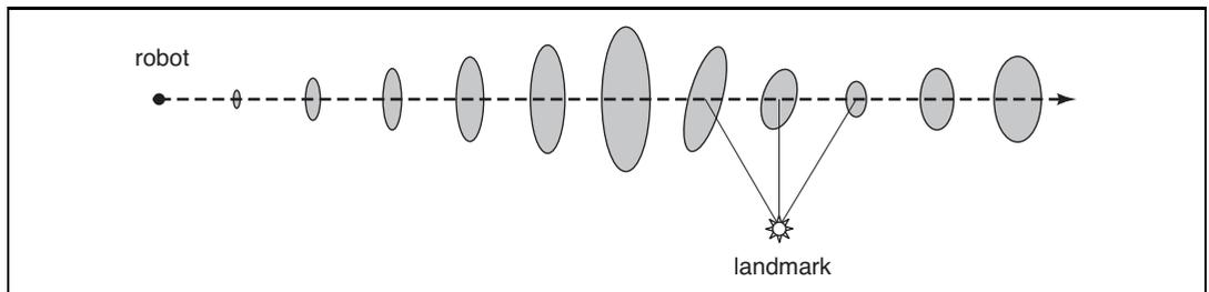
**Figure 25.12** Example of localization using the extended Kalman filter. The robot moves on a straight line. As it progresses, its uncertainty increases gradually, as illustrated by the error ellipses. When it observes a landmark with known position, the uncertainty is reduced.
