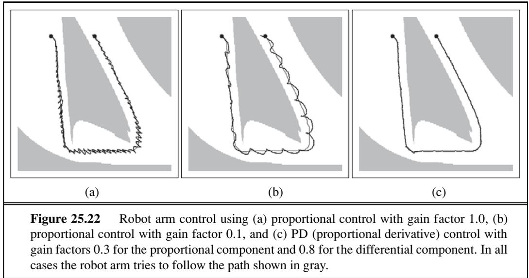
**Figure 25.22** Robot arm control using (a) proportional control with gain factor 1.0, (b) proportional control with gain factor 0.1, and (c) PD (proportional derivative) control with gain factors 0.3 for the proportional component and 0.8 for the differential component. In all cases the robot arm tries to follow the path shown in gray.
