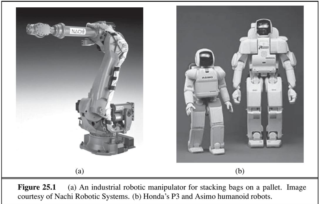
**Figure 25.1** (a) An industrial robotic manipulator for stacking bags on a pallet. Image courtesy of Nachi Robotic Systems. (b) Honda's P3 and Asimo humanoid robots.
