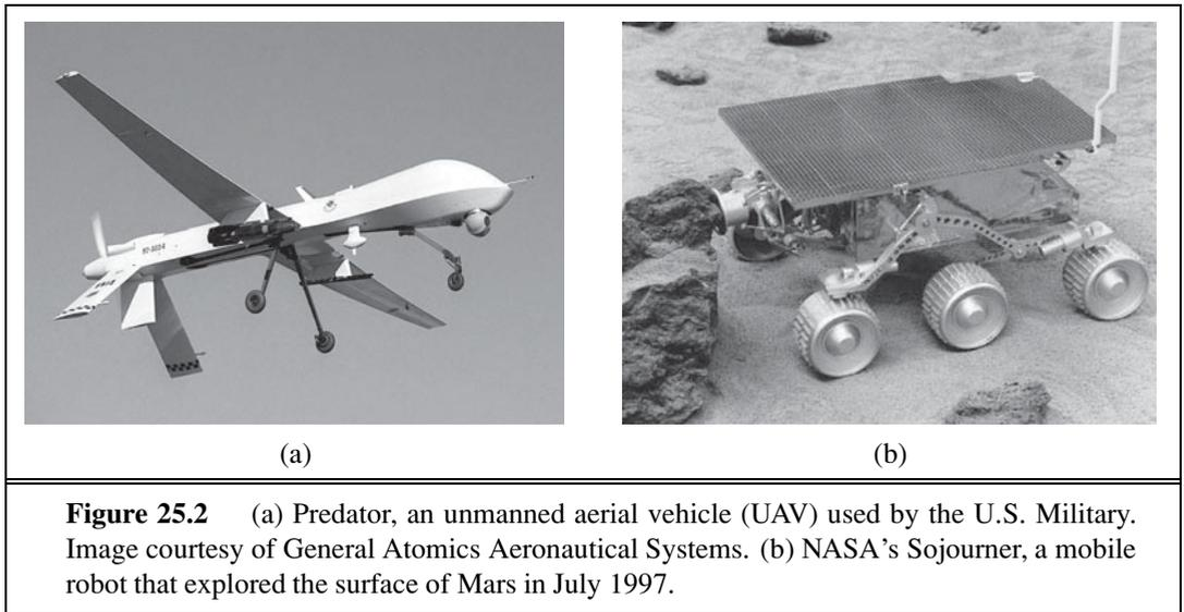
**Figure 25.2** (a) Predator, an unmanned aerial vehicle (UAV) used by the U.S. Military. Image courtesy of General Atomics Aeronautical Systems. (b) NASA's Sojourner, a mobile robot that explored the surface of Mars in July 1997.
