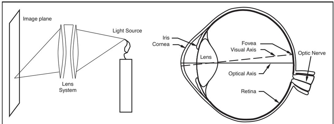
**Figure 24.3** Lenses collect the light leaving a scene point in a range of directions, and steer it all to arrive at a single point on the image plane. Focusing works for points lying close to a focal plane in space; other points will not be focused properly. In cameras, elements of the lens system move to change the focal plane, whereas in the eye, the shape of the lens is changed by specialized muscles.
