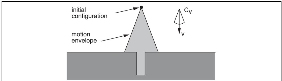
**Figure 25.19** A two-dimensional environment, velocity uncertainty cone, and envelope of possible robot motions. The intended velocity is  $v$ , but with uncertainty the actual velocity could be anywhere in  $C_v$ , resulting in a final configuration somewhere in the motion envelope, which means we wouldn't know if we hit the hole or not.
