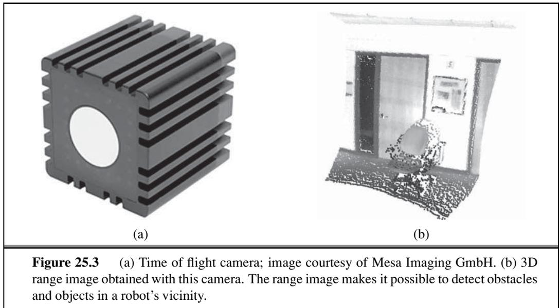
**Figure 25.3** (a) Time of flight camera; image courtesy of Mesa Imaging GmbH. (b) 3D range image obtained with this camera. The range image makes it possible to detect obstacles and objects in a robot's vicinity.
