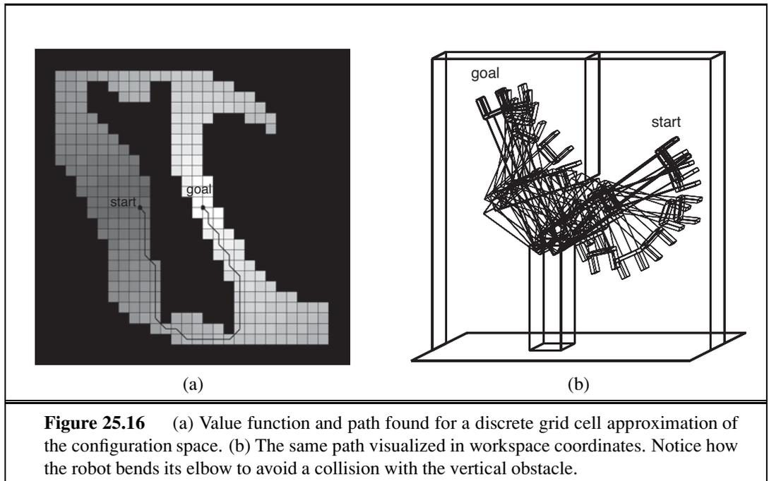
**Figure 25.16** (a) Value function and path found for a discrete grid cell approximation of the configuration space. (b) The same path visualized in workspace coordinates. Notice how the robot bends its elbow to avoid a collision with the vertical obstacle.
